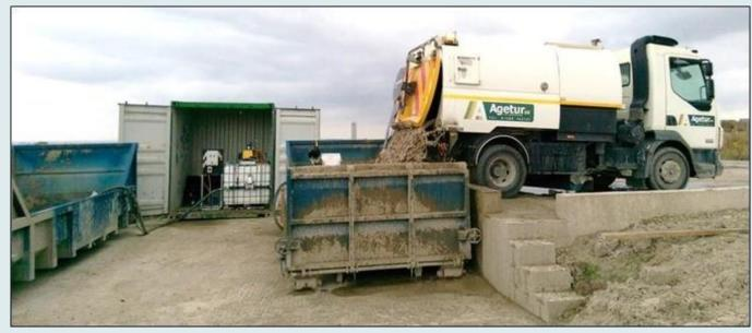
Weight: 2000kg **Length**:6m Width:2.4m Height : 1.5m Power : 5kW Water usage : No Clean water required. (Water treatment for waste water optional) **Throughput** : up to 15tph (average 10-15tph gully waste / sweepings) Loading : Direct tip with optional ramps or aggregate ramp (pictured) **Recovered products**: Dewatered product of rapidly separating solids <1mm dirty water -(Can be treated for discharge to sewer)
